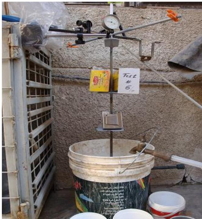
Figure (2-a): Photos showing footing assembly.
