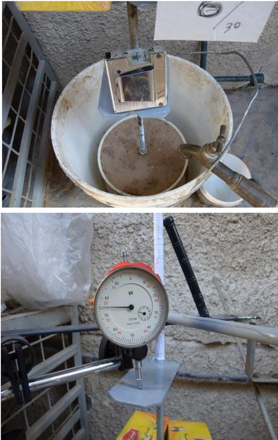
Figure (2-b): Photos showing footing assembly
